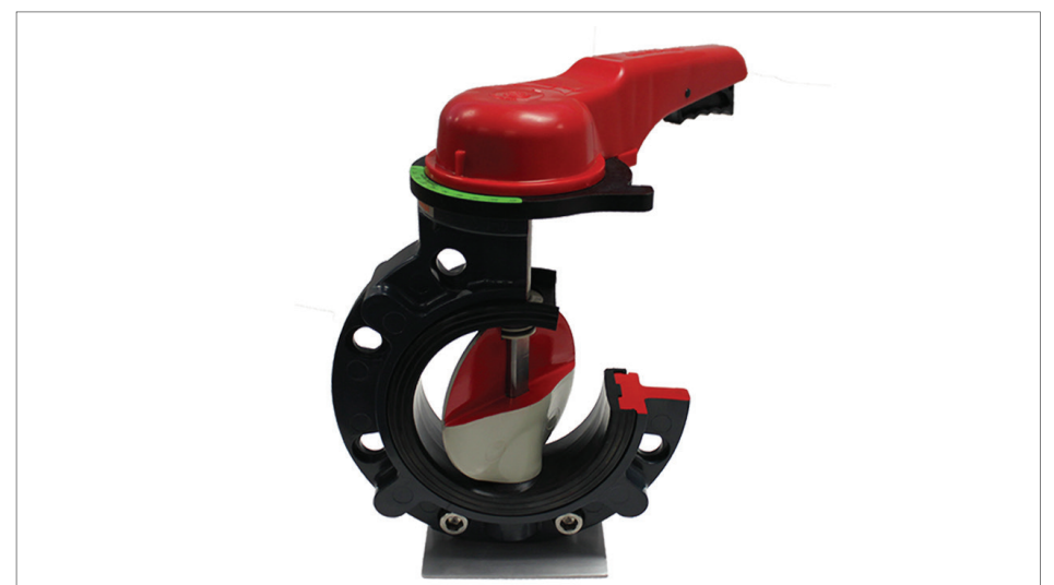
Asahi/America's Type-57 PVC butterfly valve cutaway image shows an inside look at the valve design. Over the years, Asahi has made many engineering design improvements to its butterfly valves including the spherical disk, 316 stainless steel stem, 0° to 90° green position indicator, molded valve body tag holes, increased internal sealing performance, and polypropylene stem retainer.
