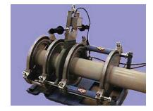
C. Watch for a continuous bead to form around both pipe ends (see pipe manufacturer or AWS/DVS standards for size). Bead must be formed 360" around each pipe.
