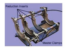
C. If necessary (e.g. T-pieces), the fixed outside clamping tool can be dismantled by unscrewing the three allen screws.
