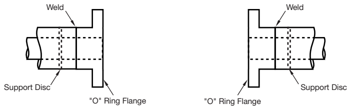
Figure F-102. Install double-wall flanges
