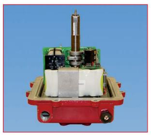
The Quarter master Protek failsafe electric actuator features a rechargeable battery pack, a built-in trickle charger, a low battery indicator, and an auxiliary limit switch that is calibrated with the fail position. The battery pack is installed inside of the actuator housing, so a separate enclosure to house the battery in not required.
