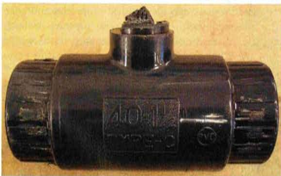
Broken valve stem due to seized ball
