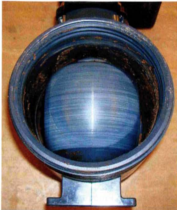
Sediment and scoring of the ball in a ball valve
