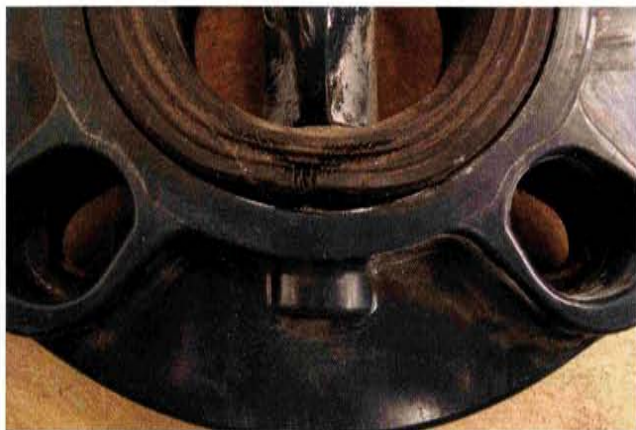
Example of a chemically attacked butterfly valve seat
